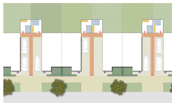
Figure 58: Illustration of cycle parking and access for semi-detached houses with on-plot parking
