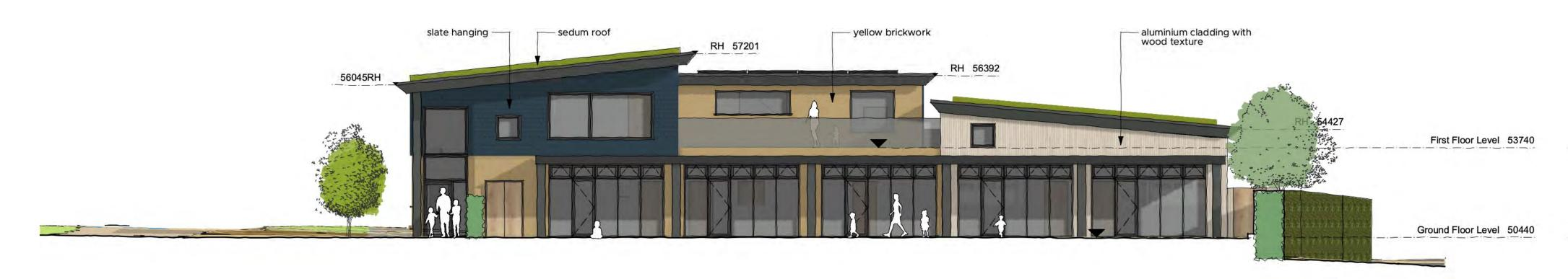
1 Proposed West Elevation Scale: 1:100
