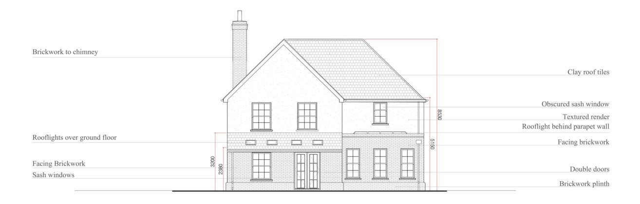
WEST ELEVATION DRAWING no. 2102. Scale 1:100@A3
