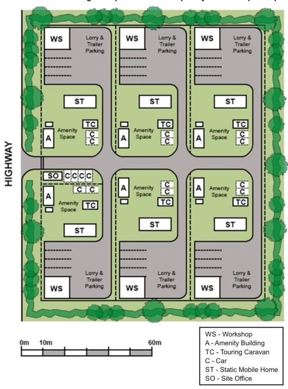
Figure 2: Indicative Travelling Showperson site example layout with shared provisions
